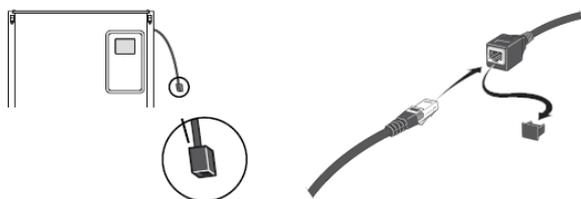
3. Insert the Ethernet cable to the cable on the backside of the system as seen on the picture above. If you have upgraded your system with NIBE Uplink you can attach the cable directly to the display as shown below.
